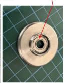
7. Put the new bearing on to the gear which is still held in the spanner, Insert into the discguard and tighten in a clockwise direction.
