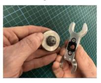
4. Carefully hold the disc with the disc removal tool and adjustable spanner. Then undo in an anticlockwise direction to remove
