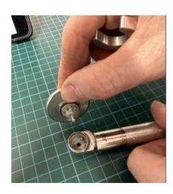
3. Using the supplied Spanner Locate onto the gear
